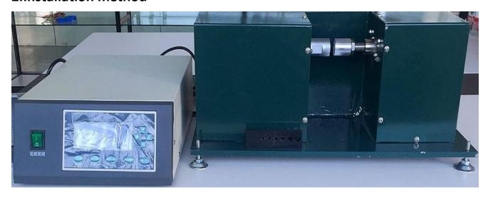
Connect the power 220V, connect the signal line plug between the power supply and the main engine.
